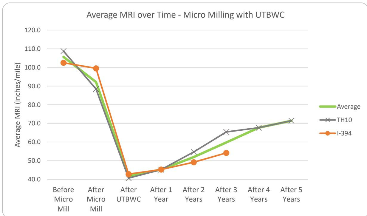
**Figure 4.09: Micro Mill and UTBWC Performance**
