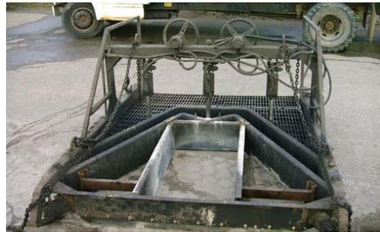
Modified micro surfacing rut box. Note the augers have been removed and a box used to straddle the longitudinal joint has been bolted into place.
